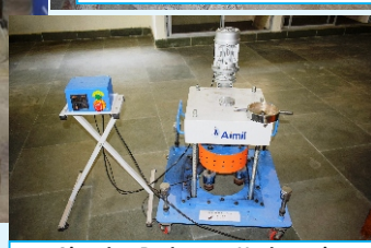
Abrasion Resistance Horizontal Concrete Surface(revolving Disk Type)
