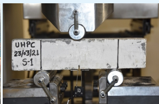
Crack Mouth Controlled Three Point Bend Testing
