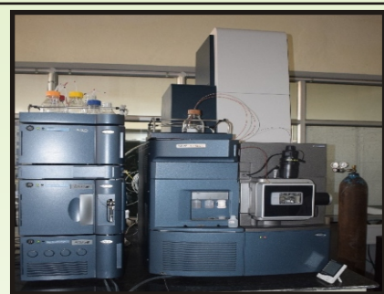
High Performance Liquid Chromatography (HPLC) with fluorescence detector Cost ₹ 256.00 Lacs
