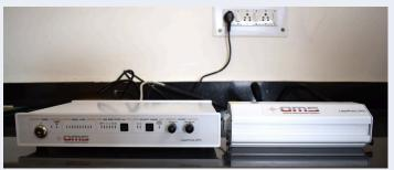
The OMS LaserPoint LP01 Laser Doppler Vibrometer is an easy-to-use precision instrument for non-contact vibration measurement of any surface. The system can be instantly used by aiming the laser beam at a target at any distance up to five meters, without the need for any optical or mechanical adjustments.
